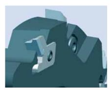
Profile knife with advanced shear angle inside.
