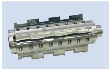
Tool example for PKS®: Multi-profiling of MDF mouldings
