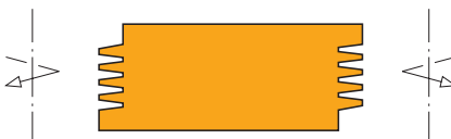
Profile 2 with staggered shoulder cutters
