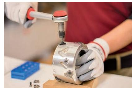
WhisperCut: Diamond knives are resharpenable in the tool body up to 3 times
