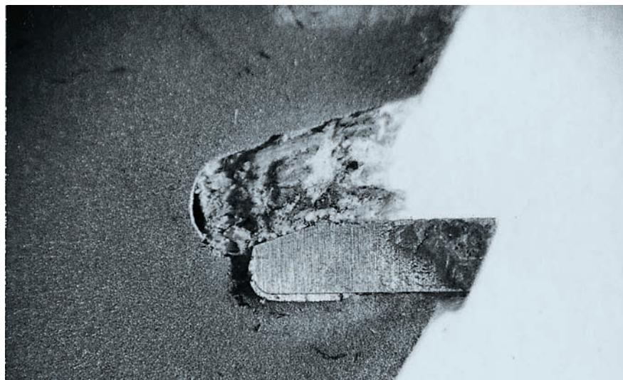
Cutting edge destruction through improper use.
