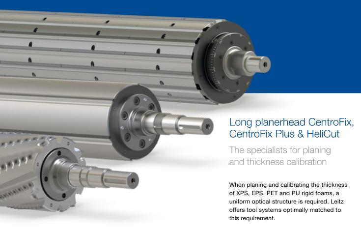
For the processing of XPS and EPS, high toothed long planerheads are recommended in order to produce surfaces with as fine pores as possible. The CentroFix and CentroFix Plus long planerheads from Leitz are optimally designed for this purpose. The tool systems achieves the best cutting results and are simple to service. The knives can be easily removed axially (CentroFix) or axially and radially (CentroFix Plus).
