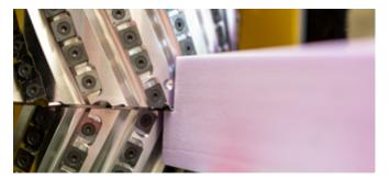
Examples for machining insulation materials – CentroFix (photo left side) for thickness calibration and HeliCut (photo right side) for lateral processing.
