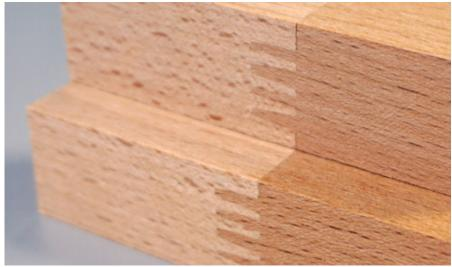
In the production of finger-joints on flat fingerjointing lines, flexible profiling, a high number of teeth and the accuracy of the finger-joint fit are among the most important requirements.
