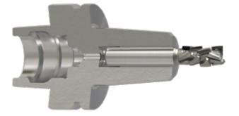
The ThermoGrip® shrink chuck is connected to the tool as if made of one piece – for low deflection and high infeed.
