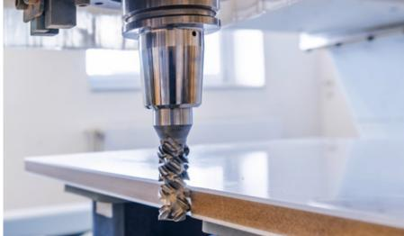
The clamping system plays a decisive role in the machining process as the interface between tool and machine. With conventional chucks, the fit clearance reduces concentricity, stability and clamping force. The result: machine and tool are not as effective as they could be.
