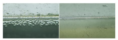
Comparison after identical running performance: The uncoated knife (left) shows heavy washouts in the carbide, while the Marathon knife (right) has an intact cutting edge and surface
