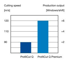
Productivity increase of up to 20% with High Speed Cutting (starting point 30 windows per shift, cutting speed 80 m/s)
