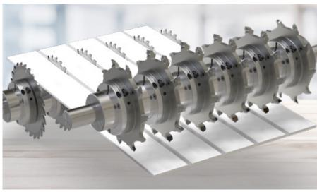
Frequently, the positioning of several tools on a single spindle is implemented by using spacers and the securing is done by a spindle nut. Due to some of the faces not being 100% square or contaminated, the shaft can become distorted. In addition, resetting to other workpiece dimensions can be very time-consuming.
