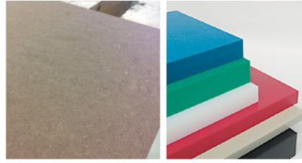
HeliPlan planing cutter: Finish quality when planing slave boards for the Nesting process (left) as well as surfaces in finish quality for thermoplastic plastic panels (right).
