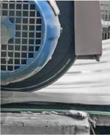
In the production of fibre cement panels, carbide-tipped circular knives for cutting the raw panels wear out particularly quickly. The consequences are a stop of the line and time-consuming tool changes.
