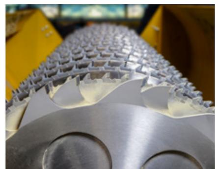
Not only the teeth, but also the gullet area of the circular sawblades are made of solid tungsten carbide and thus effectively prevent washing out of the tool body. This results in excellent durability and a maximum tool life.
