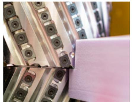
The HeliCut system is perfect for the side processing of insulation panels.
